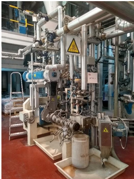
Extrusion process for feed prototypes production
